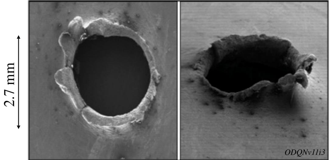
Cause: Grain of fiber glass, 1.2 mm, 2 mg, Mach 12.
