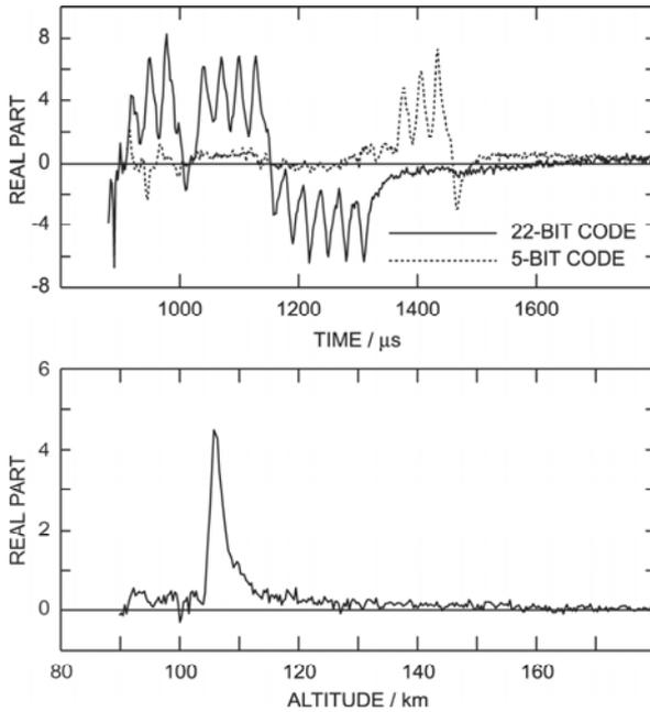
Figure 6. Top: Height profiles of the real part of the 30-s lag for the applied 22-bit and 5-bit codes. Bottom: The corresponding lag profile obtained means of the inversion method.
