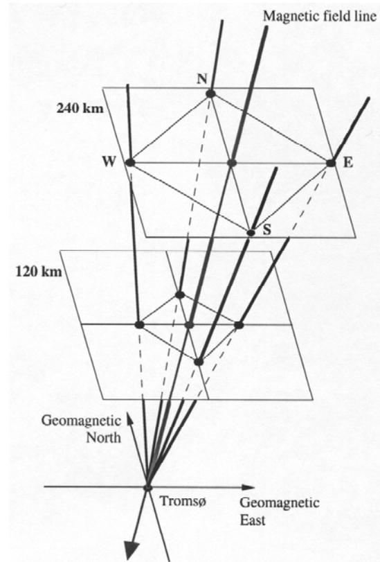
Figure 14. The scanning arrangement, with squares of 50 and 100 km on a side in the F-layer. Each scan takes 10 minutes throughout which a steady state ionosphere is assumed.
