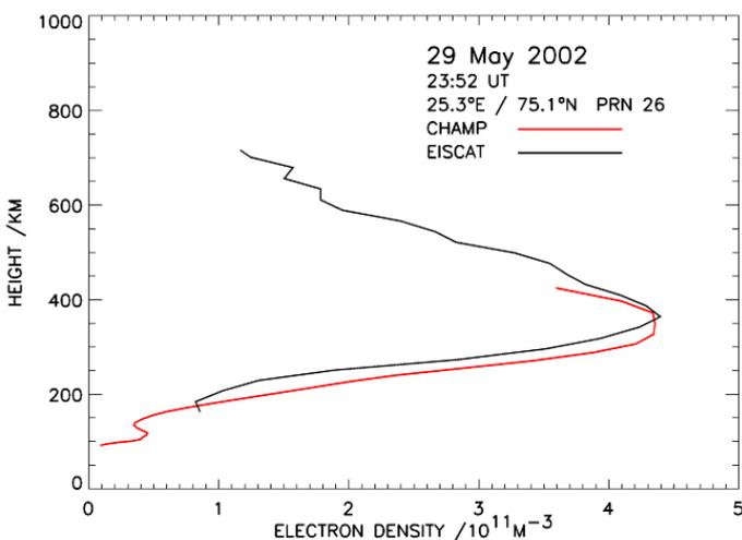
Figure 11. Electron density profiles from CHAMP-GPS reconstruction (red) and the EISCAT UHF radar (black) where the long pulse data from the cp1t modulation was used.
