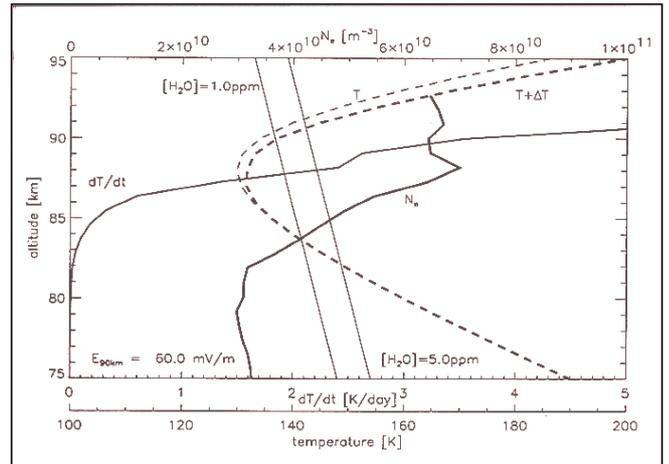
Figure 9 Height profiles of measured electron density  $N_e$ , heating rate  $dT/dt$ , neutral temperature  $T$  before and after the Joule heating (dashed lines), and the limiting water vapour mixing ratio.
