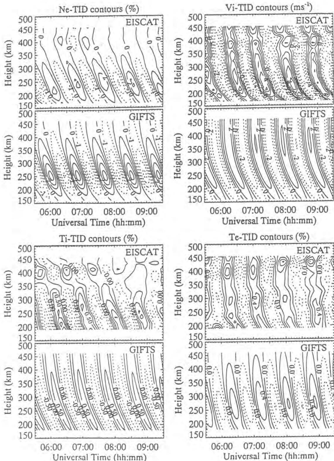
*Fig. 52. One-to-one comparison of modelling results (labelled 'GIFTS') to EISCAT data (labelled 'EISCAT') for a TID event on August 31, 1988. Comparisons for the set of TID quantities ( $dNe/Ne_0$ ,  $dVi$ ,  $dTi/Ti_0$ ,  $dTe/Te_0$ ) are shown.*
