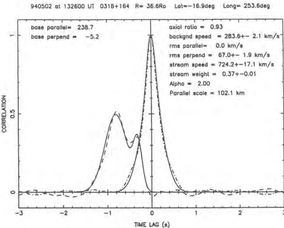
*Fig. 1(b) Correlation functions for 0318+164 on 2 May 1994 fitted using the two-velocity model. Observed correlation functions are shown as dashed lines, model fits as solid lines.*
