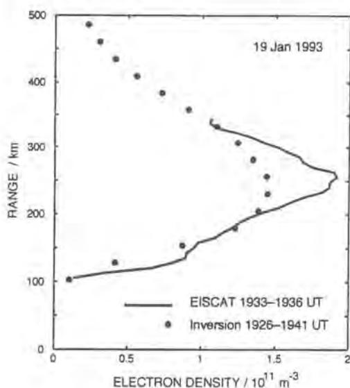
*Fig. 28. Comparison of  $N_e$  profiles deduced from satellite radio-tomography and measured by the EISCAT radar.*
