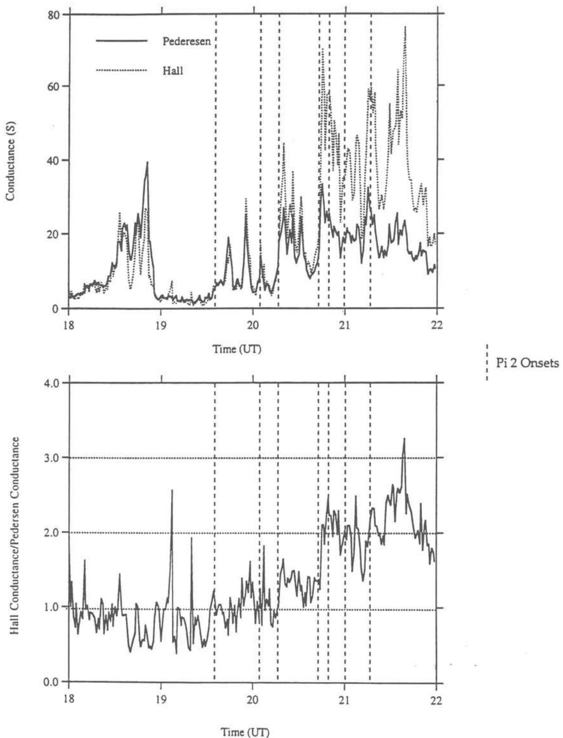
Fig. 37. In the top panel the Pedersen (solid line) and Hall (dotted line) Conductances are plotted as a function of UT from 18:00 to 22:00 UT. The lower panel shows the ratio of Hall to Pedersen Conductance for the same interval. The dashed vertical lines in each panel represent the times of Pi2 pulsations.
