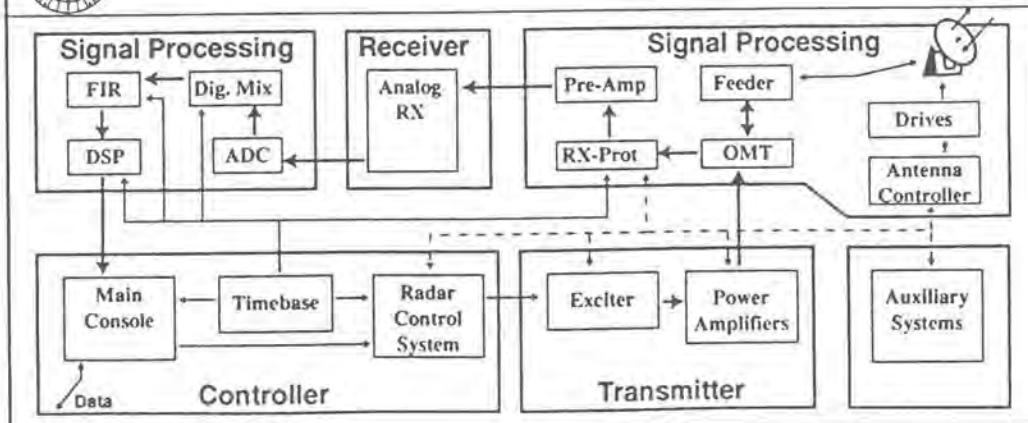
The block diagram shows the main instrument components of the ESR system, which had been set up at the site during the past three years. Controller, receiver, signal processing and other accessory equipment are located in the control room, the transmitter in the large transmitter hall, and the antenna just adjacent to the building.
