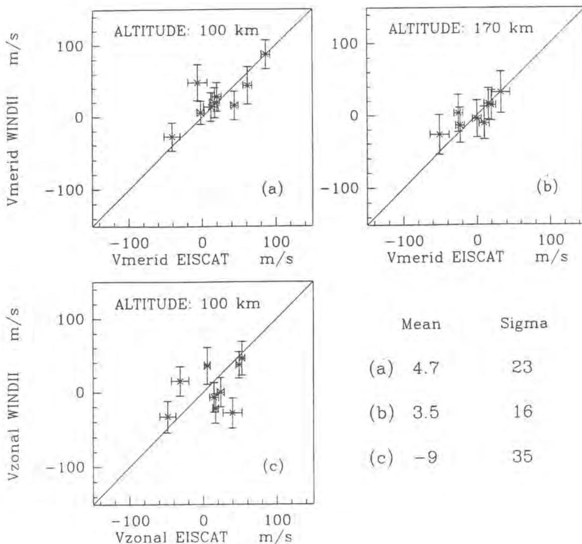
Fig. 48. Scatter plots for WINDII-EISCAT meridional (panels a and b) and zonal (panel c) winds comparisons. For each panel, the mean difference WINDII-EISCAT is indicated with its standard deviation.
