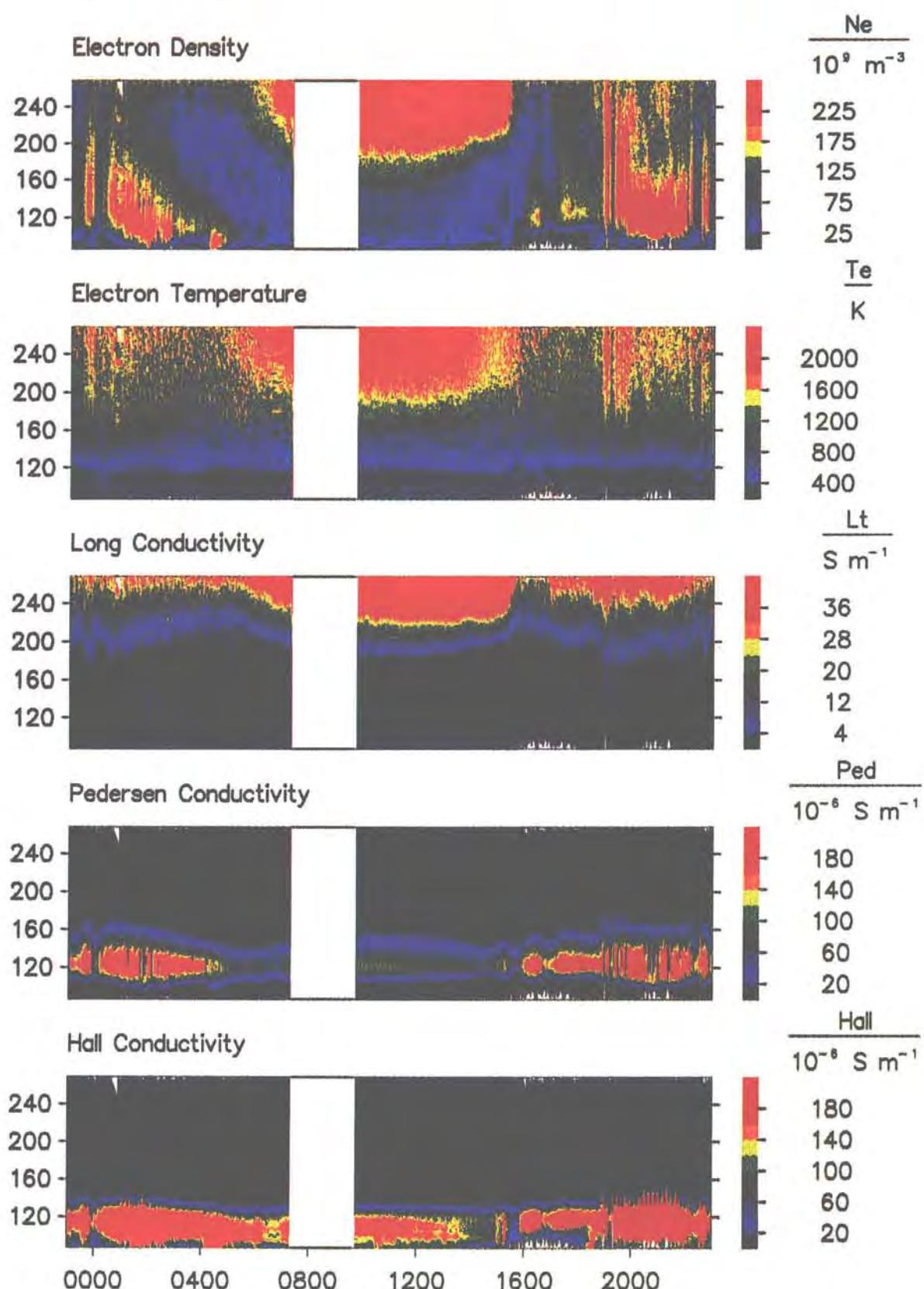
Fig. 38. Height-time plots showing ionospheric conductivities. As well as the diurnal quiet-time variation, the effects of disturbances are seen around 01 UT and 21 UT.
