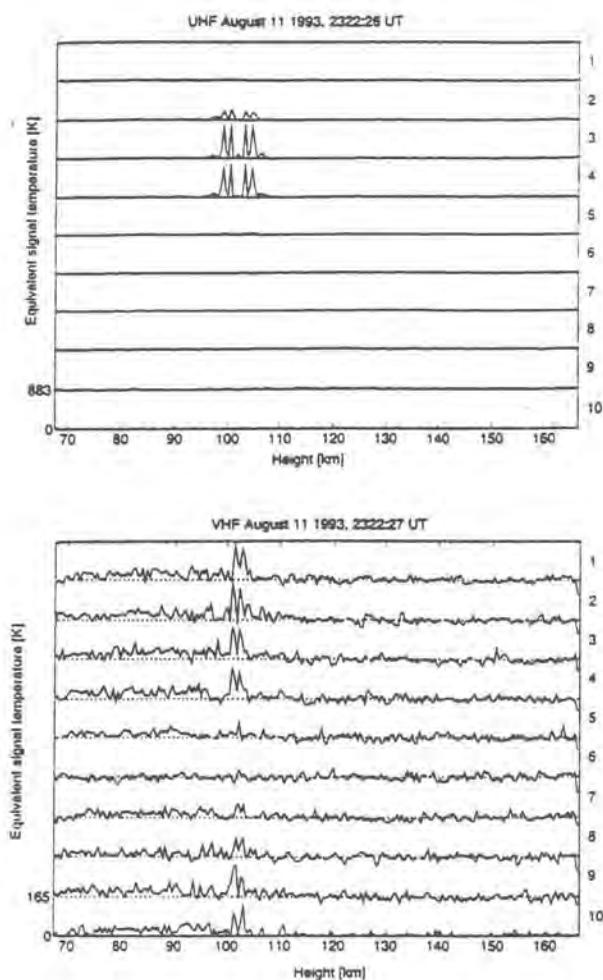
Fig. 35. A time-resolved dual radar meteor event from the Perseid operation on August 11, 1993, UHF data (a) and VHF data (b). The velocity fits yield  $17.4$  and  $17.5 \text{ km s}^{-1}$  respectively, showing that this is probably a sporadic meteor rather than a shower.
