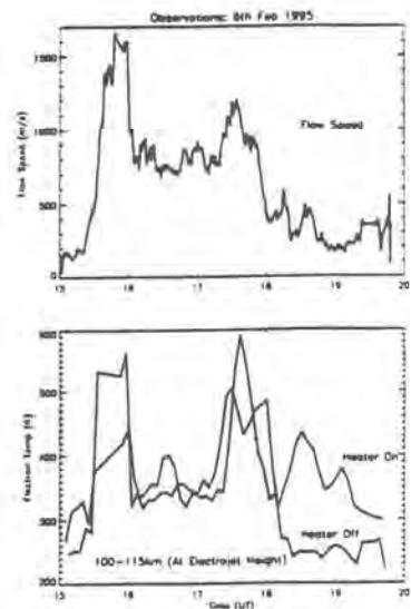
*Fig. 6. EISCAT measurements of the F-region plasma flow speed (top panel) and the electron temperature in the E-region (100 - 115 km) during intervals when the heater was off or on.*
