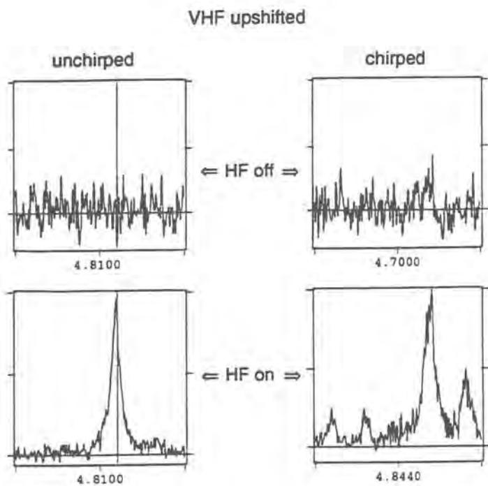
Fig. 9(a). Upshifted plasma line spectra measured with the VHF radar. The vertical axis is self-normalised spectral power in arbitrary units. The horizontal axis is frequency covering a bandwidth of 1 MHz. The top panels were measured during a heater off cycle of 2 s and the bottom panels during the previous cycle with heater on. The transmitter pulse was not chirped for the left panels while it was for the right.
