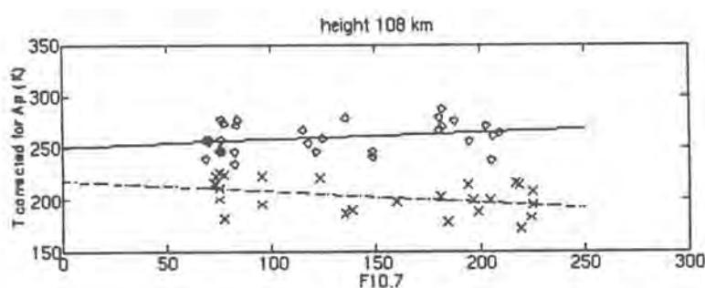
Fig. 49. Variation of daily average temperatures from EISCAT CP-1 and CP-2 experiments, at 108 km altitude, as a function of solar activity: o for summer, x for winter.
