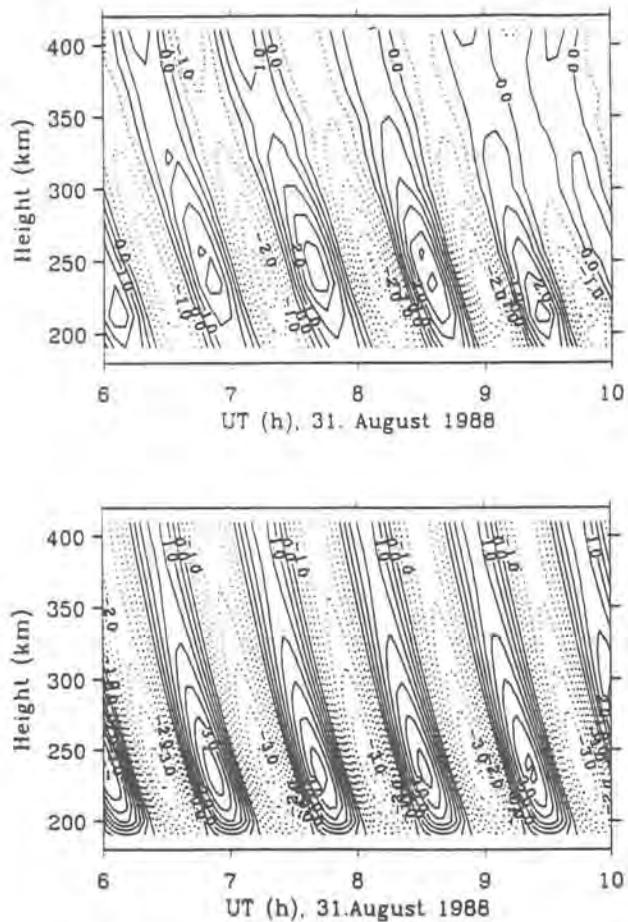
Fig. 51. Height-time amplitude contours of the TID quantity  $dNe/Ne_0$  [%]. The modelled Ne-TID (lower panel) is compared with the Ne-TID in EISCAT data measured at August 31, 1988 (upper panel; bandpass filtered with a central period of 50 min.)
