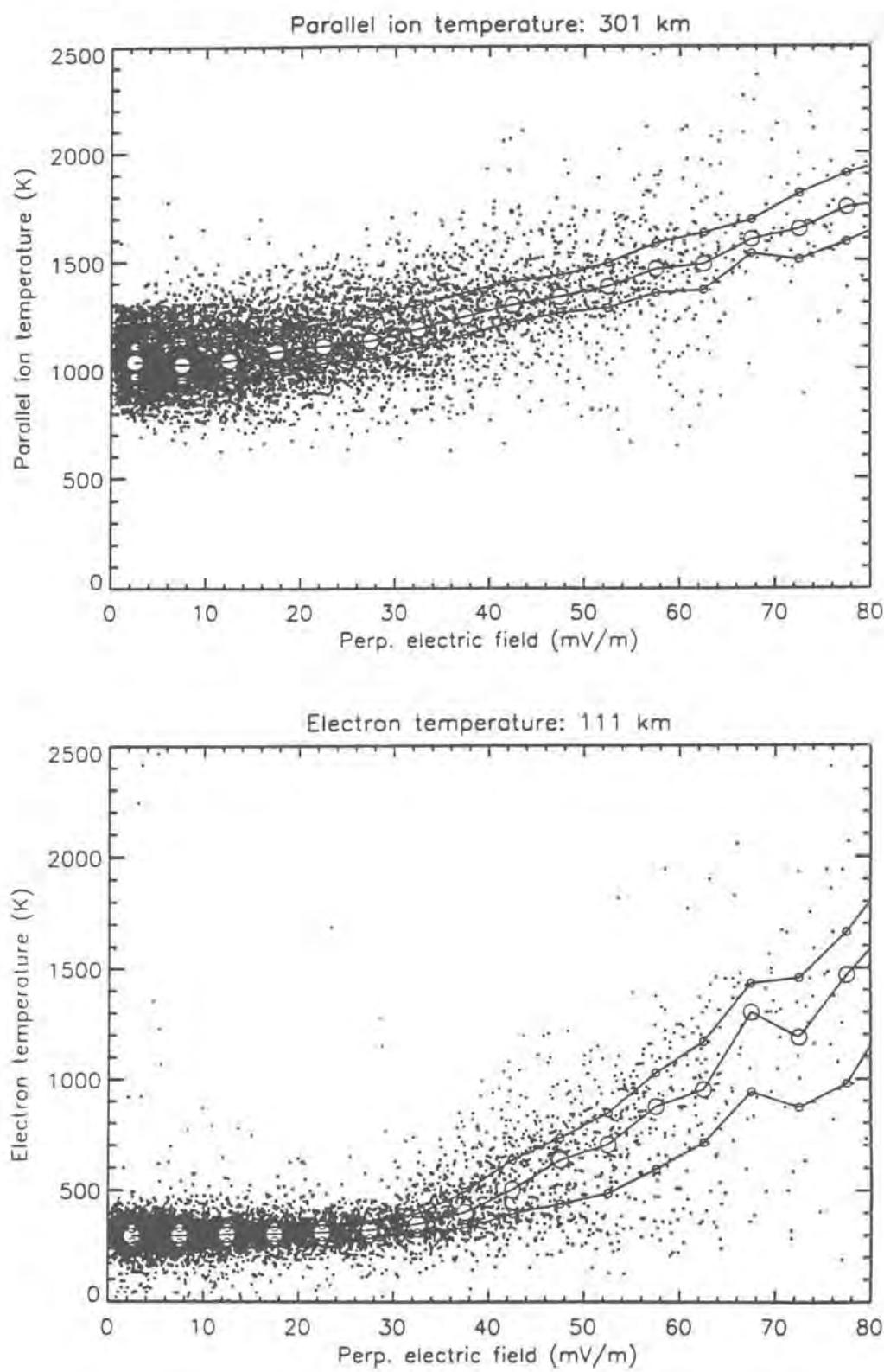
Fig. 34. The measured parallel ion temperature as a function of the perpendicular electric field measured by EISCAT CP-1 and CP-2 experiments from 1990 - 1995. Simultaneous measurements of the electron temperature at 111 km as a function of the perpendicular electric field are given in the bottom panel.
