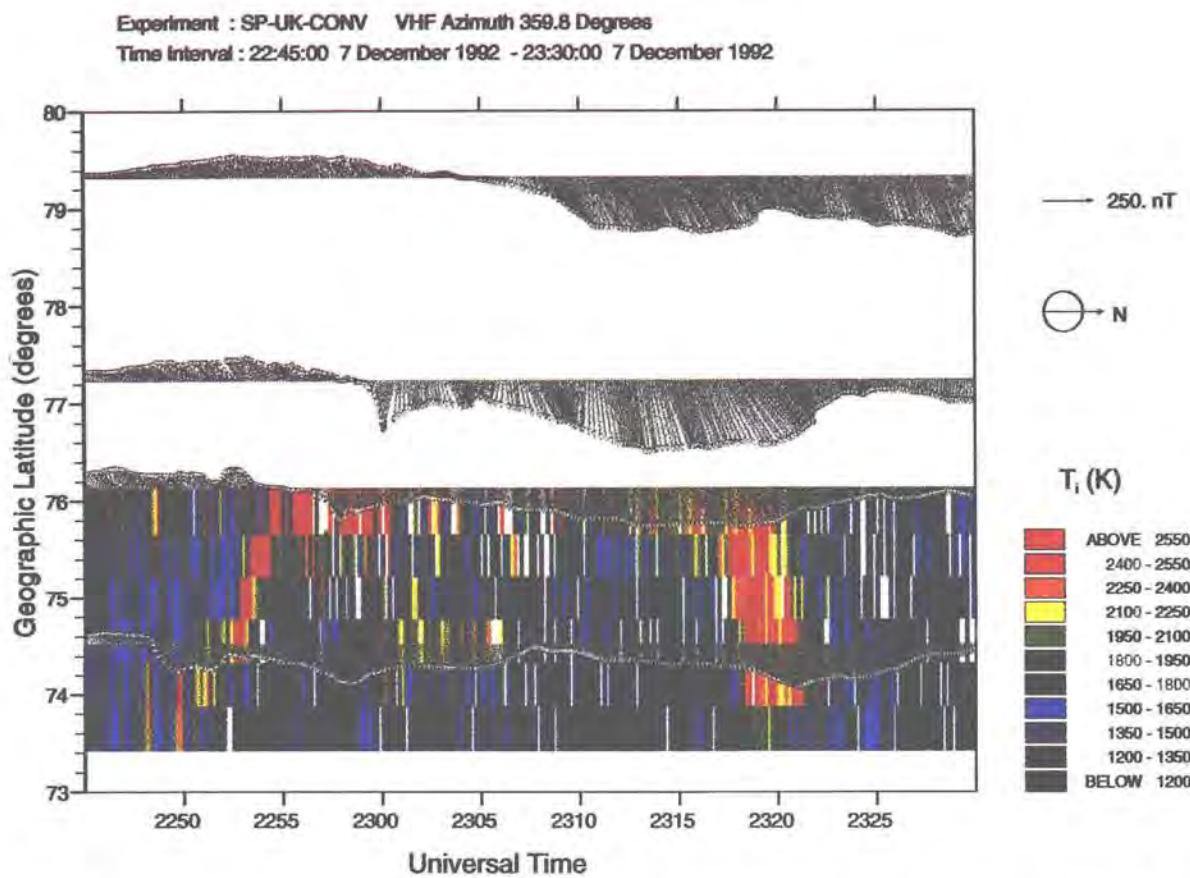
Fig. 46. EISCAT observations of ion temperatures and magnetic perturbations detected by local IMAGE magnetometers on Svalbard, observed in a major multi-instrument study of a substorm during the second Earth fly-by of the Galileo satellite. The data reveal a separate electric field and current system poleward of the main substorm electrojet.
