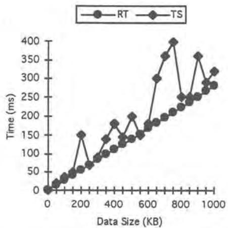
Data transfer tests for the DSP system, demonstrating the advantage of running real-time (RT) with respect to timesharing (TS). The lower block diagram shows the principle of the digital receiver and the photos some actual components.
