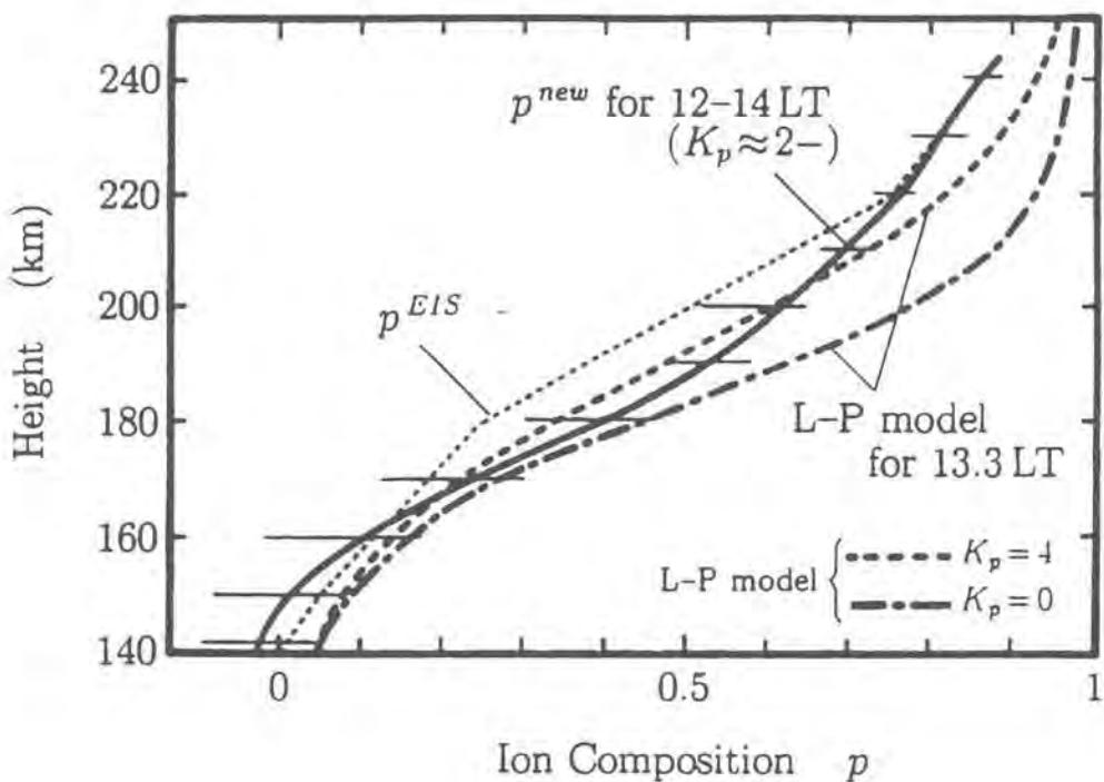
Fig. 24. New ion composition model for 12-14 LT as compared to the summer model for 12 UT (approx. 13.3 LT) of Lathuillere and Pibaret (1992). The horizontal bars attached to the  $p^{new}$  curve denote the deviation range among the 8 sample profiles available in the interval 12-14 LT. The thin dotted line represents the standard model.
