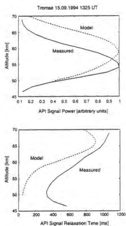
*Fig. 8. Comparison between the measured and model values of signal relaxation times (upper panel) and relative signal power (lower panel) for the API experiment at Tromsø on 15 September, 1994, 1325 UT.*
