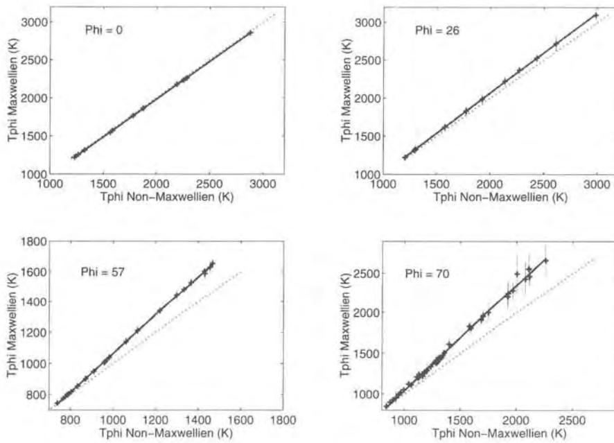
Fig. 31. Line of sight temperature of  $\text{NO}^+$  ions obtained by the standard EISCAT analysis as a function of the line of sight temperature obtained with non-Maxwellian analysis. Each panel corresponds to a different aspect angle ( $\phi$ ) and allows quantification of the  $\text{NO}^+$  line of sight temperature overestimation, when the standard EISCAT analysis is used.
