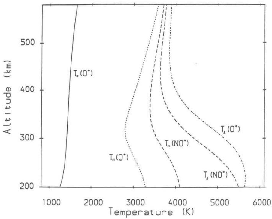
Fig. 22. Model ion temperatures as a function of altitude at 50 minutes elapsed time during the heating event of 5 September 1989. The continuous line represents the altitude variation of the field-parallel  $O^+$  temperature before the start of the event.
