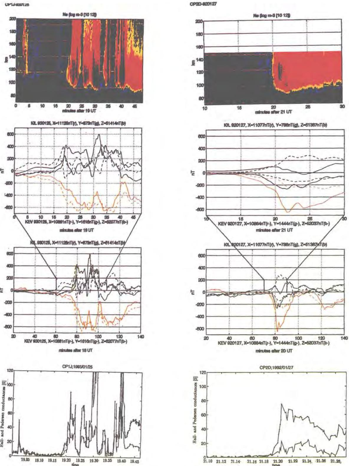
Fig. 47. Electron density in the E-region measured by EISCAT (top), nearby geomagnetic variations (centre two panels) and derived conductivities (bottom) for a local substorm onset (right column) and a westward travelling surge (left column).
