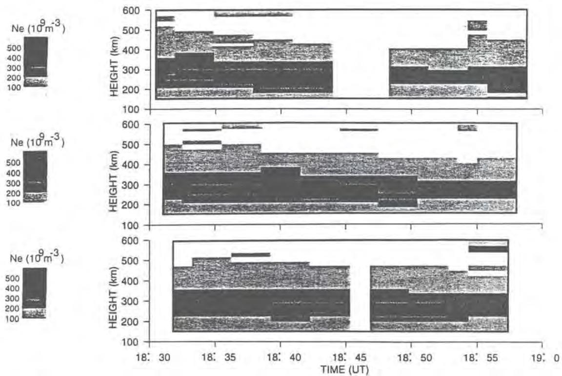
*Fig. 26.* EISCAT long pulse electron density contours on 23 May 1994. The panels, from top to bottom, correspond to beam elevations  $96^\circ$  (north),  $90^\circ$  and  $84^\circ$  (south). An F-region feature is seen first in the top panel at 18:36 UT. It then moved southwards through the other two positions, finally disappearing at around 18:50 UT.
