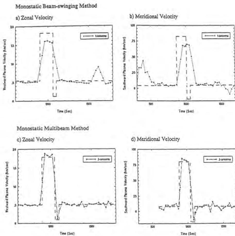
Fig. 13. A comparison of the simulated results obtained by a monostatic single-antenna beam-swinging method and a monostatic three-antenna multibeam method when observing an auroral arc drifting over the radar.
