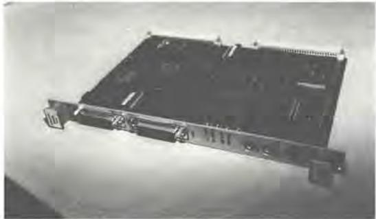
The digital signal processing (DSP) includes the on-line computation of both full autocorrelation lag profiles and frequency power spectra, handling all required modulations coded in amplitude and phase. The DSP system is designed and programmed using modified commercially produced DSP boards.
