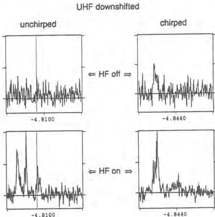
Fig. 9(b). Down-shifted plasma line spectra measured with the UHF radar. See (a) for additional explanation. The measurements shown in (a) and (b) were taken simultaneously.
