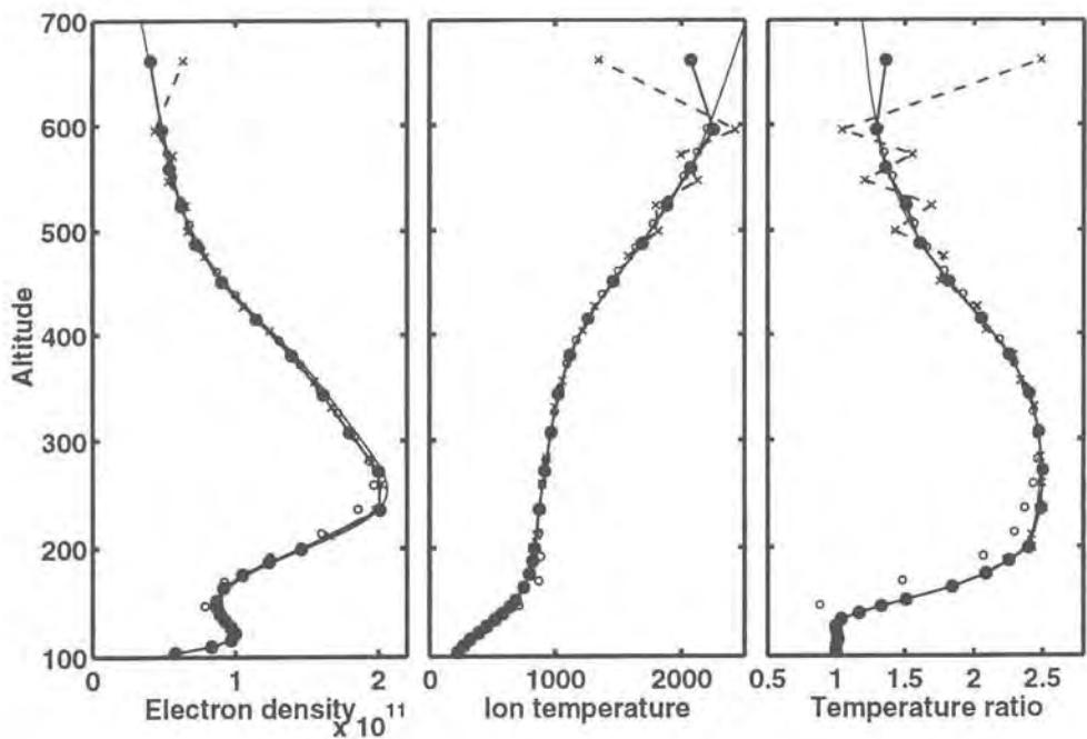
Fig. 10. Full profile analysis results (full circles) of EISCAT UHF data measured on February 16, 1993, at 1110--1140 UT. The parameter grid spacing is 6 km below the 150 km altitude, 12 km up to the 200 km altitude, and 30 km above the 200 km altitude. The gated analysis results of the long pulse data by the open circles.
