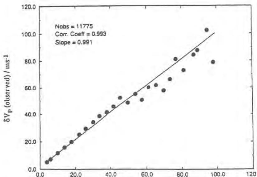
Fig. 12. Relationship between the predicted and observed values of the rms error in measuring plasma velocity (data analysed by the full-fit method).
