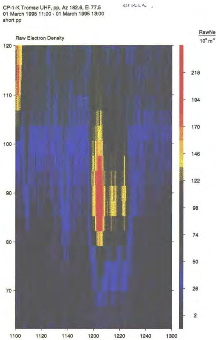
*Fig. 56(b)* Colour representation of EISCAT electron densities from CP-1 power profile measurements on 1 March 1995 as the absorption event shown in Fig. 56(a) crossed the radar beam. Note the low altitude of the peak (about 88 km) and that a density increase was seen even in the lowest range gate (62.2-65.3 km altitude), indicating the presence of electrons with energies of at least 300 keV.
