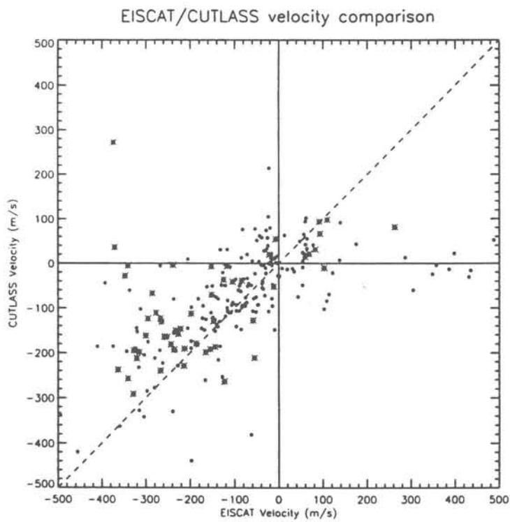
Fig. 23. Scatter plot of EISCAT ion velocity and CUTLASS irregularity drift velocity measurements.
