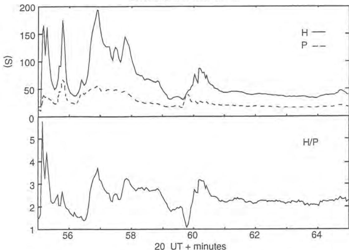
Fig. 39. Hall (solid line) and Pedersen (dashed line) conductances (top panel), and the Hall to Pedersen conductance ratio (bottom panel) obtained by 3 s integration during the expansion phase of a substorm. The highest conductances are observed at the edges and inside of a WTS.
