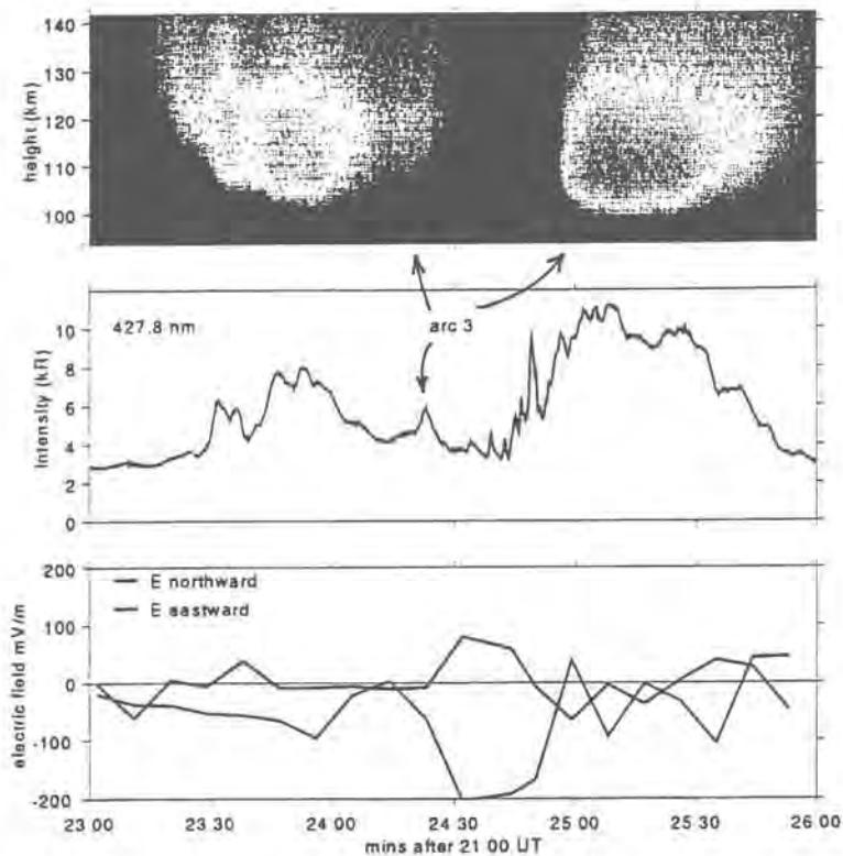
Fig. 42. ElSCAT electron density profiles at 0.2 s resolution with maximum density greater than  $10^{12} \text{ m}^{-3}$  (top panel). Photometer measurements with wider field of view than ElSCAT, showing the fast temporal variation at 21:24:30 in 'arc 3' (middle panel). Horizontal electric field measurements at 9 s resolution (bottom panel).
