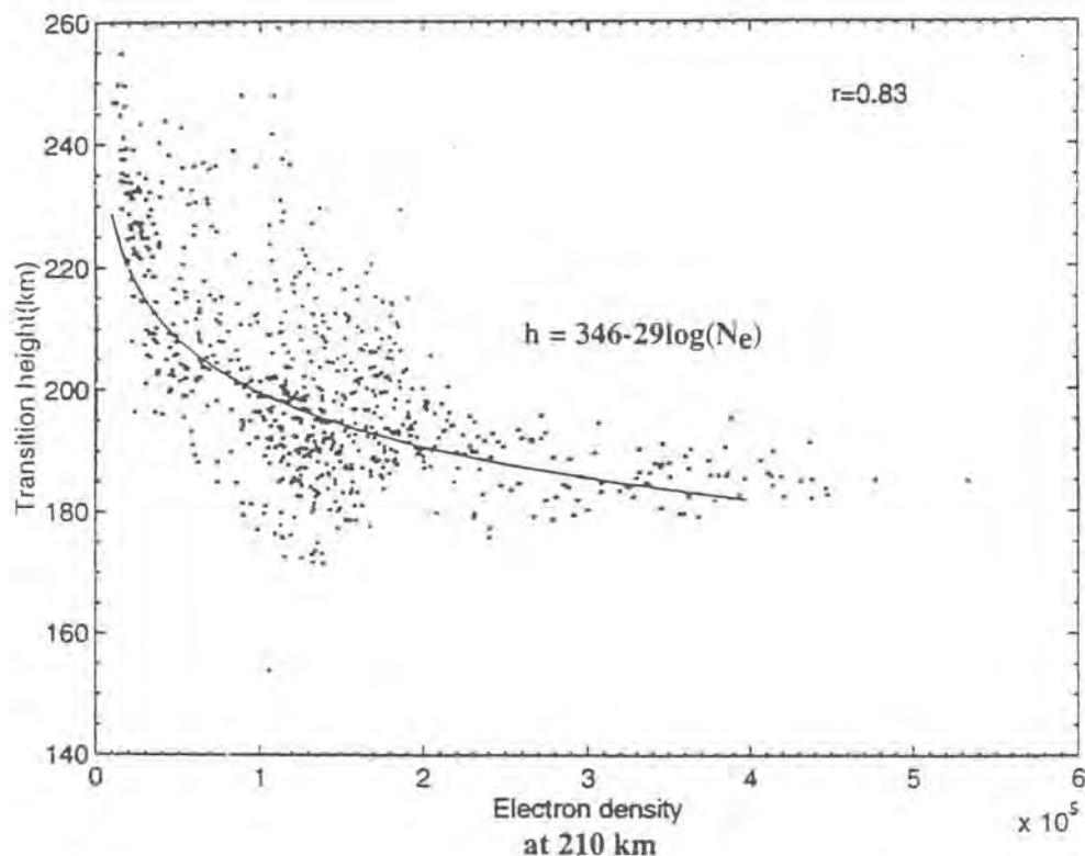
Fig 25. The altitude with an ion content of 50%  $O^+$  as a function of electron density at 210 km together with the best fit. The error bars (omitted) are higher for lower densities.
