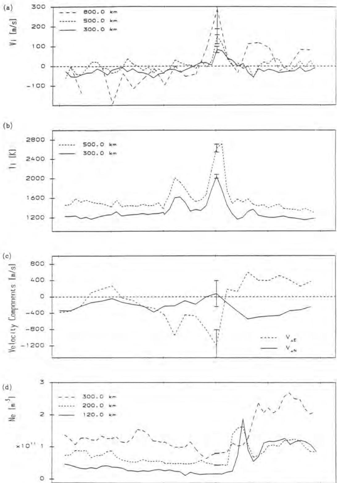
Fig. 19. EISCAT observations from 17 January 1990; (a) Line-of-sight (vertical) ion velocities measured by the UHF (300 and 500 km) and VHF (800 km) radars; (b) Line-of-sight ion temperature at 300 and 500 km altitude measured by the UHF radar; (c) Zonal and meridional components of plasma drift velocity, calculated from tristatic observations at 315 km; (d) Electron density at 200 and 300 km (from long-pulse) and at 120 km altitude (from power profile).
