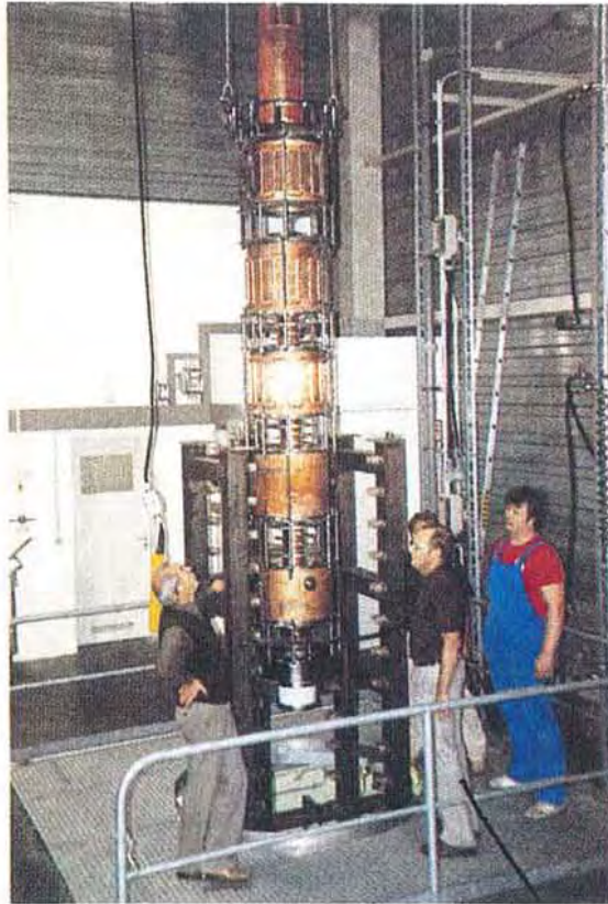
Figure 12: VALVO VHF Klystron on hoist before positioning in bake-out station. The tube is more than 5 metres long and is designed to produce 3 Mw of peak pulse power.
